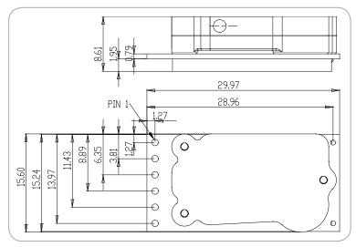
All dimensions in millimeters (mm)
